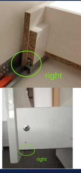
Step 1. Make sure the metal hooks on the sliders are properly inserted into the pre-drilled holes on both sides of drawer.
