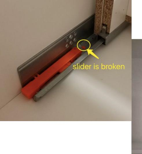
Step 3. Check if the rebound device is in good condition. If rebound device has separated from the slider, then the slider must be replaced.
