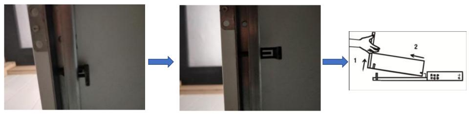
STEP 1 Pull out the black button on the two sides of the sliders at the bottom of the drawer at the same time. STEP 2 Lift the drawer to remove the drawer.
